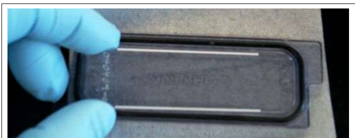
Placement of slide and cover slip, assembled, into a hybridization chamber base
