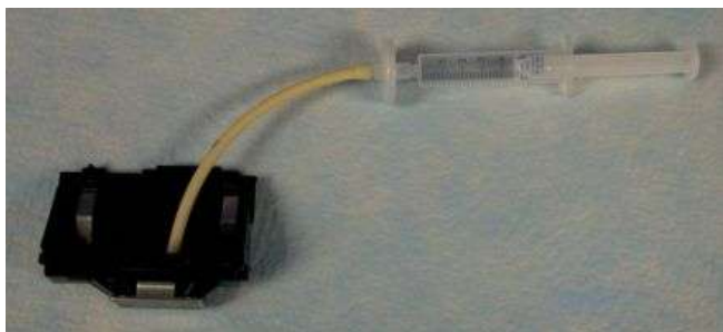
Syringe, filter, and tubing used for flushing out packing material prior to installation of the new inkjet head on the POSaM instrument.
