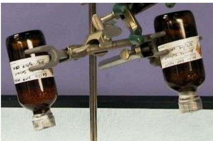
Storage of solvent in inverted, parafilm-sealed bottles.
