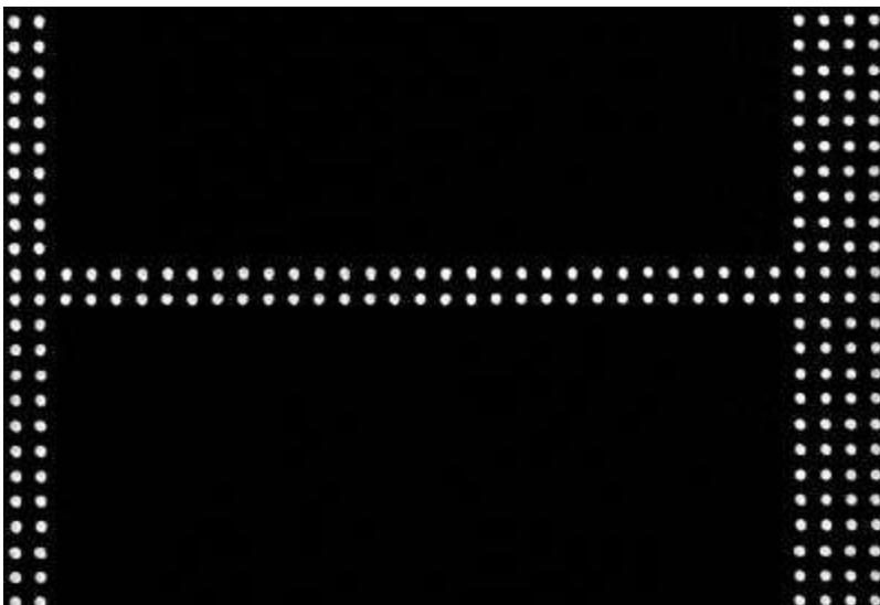
Portion of a control border scanned with standard settings, illustrating round, uniformly spaced features indicative of a good array printing
