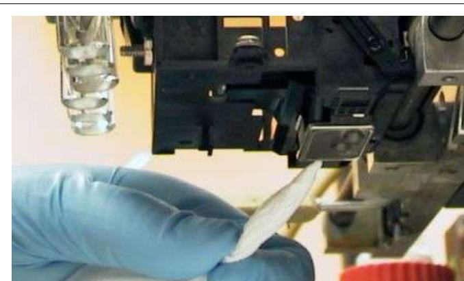
Hanging drops being removed with a Kimwipe from underside of inkjet head
