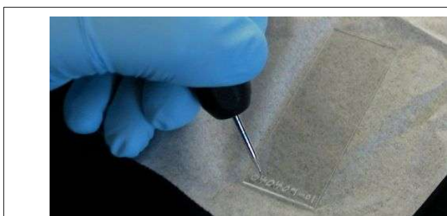
Engraving of Unique Identifier on slide prior to loading; standard format is YYMMDD-nn
