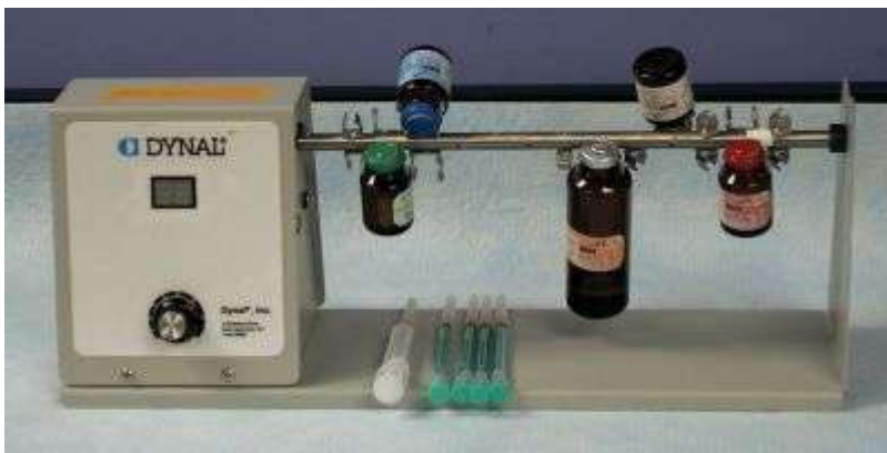
Prepared phosphoramidites and Tetrazole on the rotary mixer.
