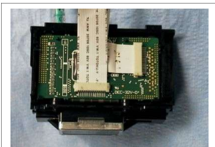
Connection of ribbon cables to the circuit board on the backside of the inkjet head prior to installation
